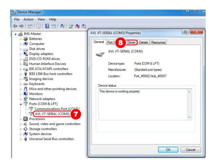
STEP 07: Go to AVL VT SERIAL under options Ports (COM & LPT) and make double click on it STEP 08: Go to tab Driver
